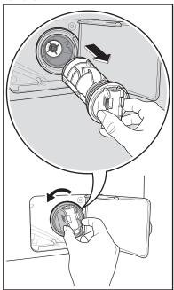
**6.** Remove fluff and objects from the pump filter (if there are any).
