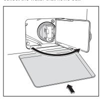
**3.** Press the two levers and pull forward the drainage duct to let the water flow out.
