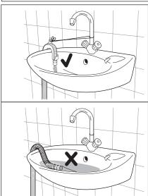
In this case, make sure the end cannot come unhooked when the machine will be emptied. This could be done by tying it to the tap with a piece of string or attaching it to the wall.
