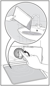
Pull back the drainage duct and turn the filter counter-clockwise to remove it.
