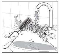
Make sure that the impeller of the pump can turn. If this does not occur, contact the service centre.
