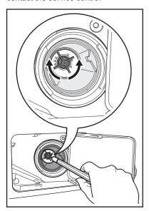
9. Put the filter back in the pump.
