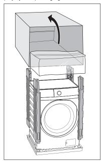
Open the door. Remove the polystyrene piece from the door seal and all the items from the drum.
