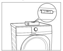
If you do not have a spirit level, as a guide use the edge of a door frame, cupboard or bench to check that the Washer-Dryer is leveled.
